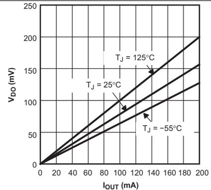
Figure 12. Dropout Voltage vs Output Current
