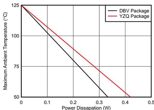
**Figure 24. Maximum Ambient Temperature vs Power Dissipation**
