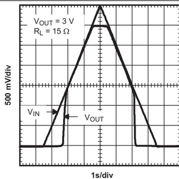
Figure 11. Power Up and Power Down
