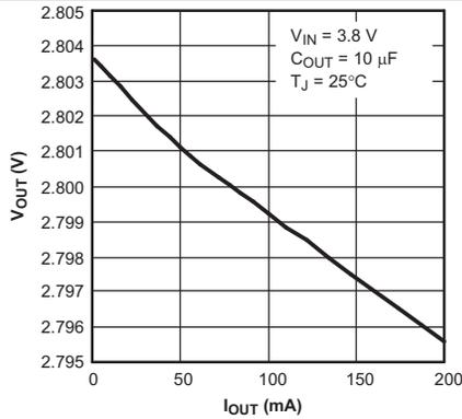
Figure 1. TPS73028 Output Voltage vs Output Current
