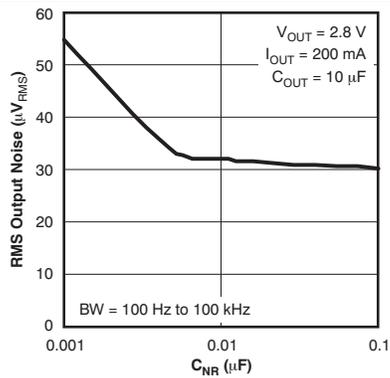
Figure 5. Root Mean Square Output Noise vs  $C_{NR}$
