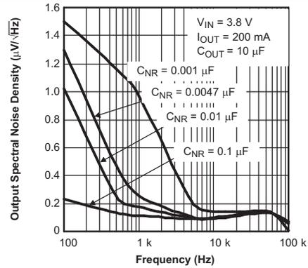
Figure 4. TPS73028 Output Spectral Noise Density vs Frequency
