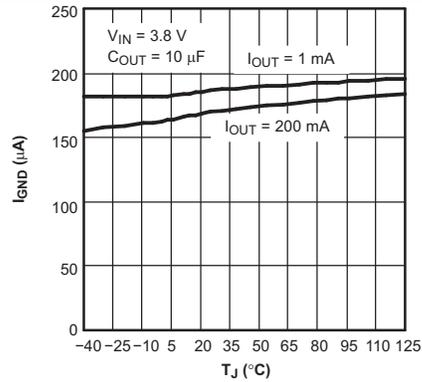
Figure 3. TPS73028 Ground Current vs Junction Temperature
