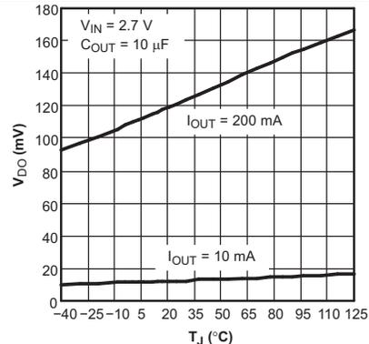
Figure 6. TPS73028 Dropout Voltage vs Junction Temperature
