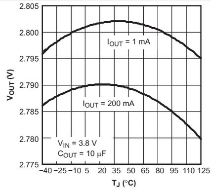
Figure 2. TPS73028 Output Voltage vs Junction Temperature
